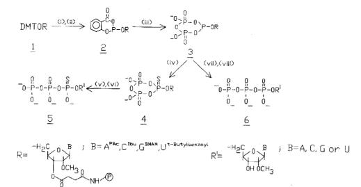
Scheme 1. Reagents and conditions: (i), 3% TCA in CH<sub>2</sub>Cl<sub>2</sub>; (ii), salicyl phosphorochloridite; (iii), 0.5 M bis-tri-n-butylammonium pyrophosphate in DMF and tri-n-butylamine; (iv), sulphur; (v), dioxan-water; (vi) & (viii), 25% aq. ammonia; (vii), Iodine-waterpyridine-THF; PAc=phenoxyacetyl; Ibu=isobutyryl; DMAM=dimethylaminomethylidene, P=polymer support, DMT=4,4'-dimethoxytrityl.
